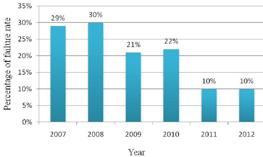
**Figure 11: Failure Rates of 2000 Certification Projects for IEC 61215**
