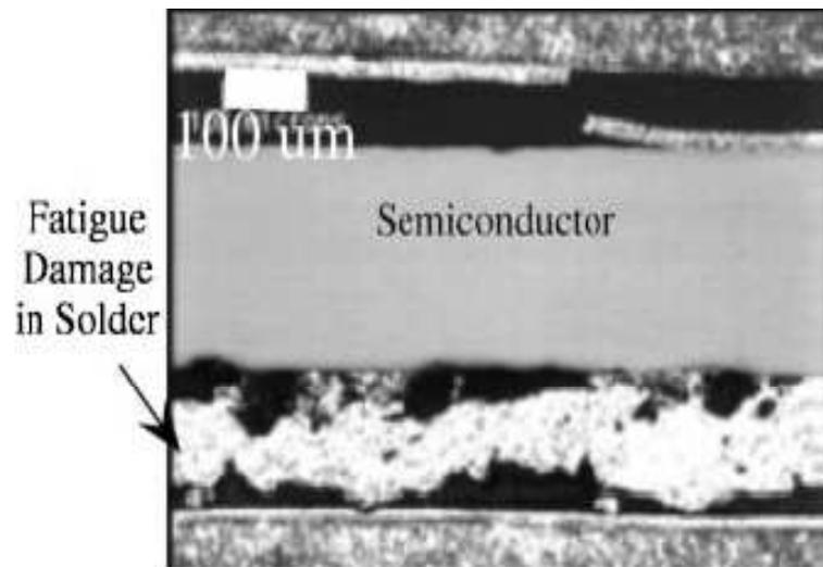
**Figure 5: SEM Image of Snpb Solder PV Cells Subject to Long-Term Field Exposure Showing Significant Solder Fatigue Damage [4]**
