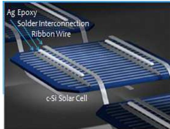
**Figure 3: Schematic of Solder Interconnection between Ribbon Wires and Wafer-Based Crystalline Silicon Solar Cells [8]**
