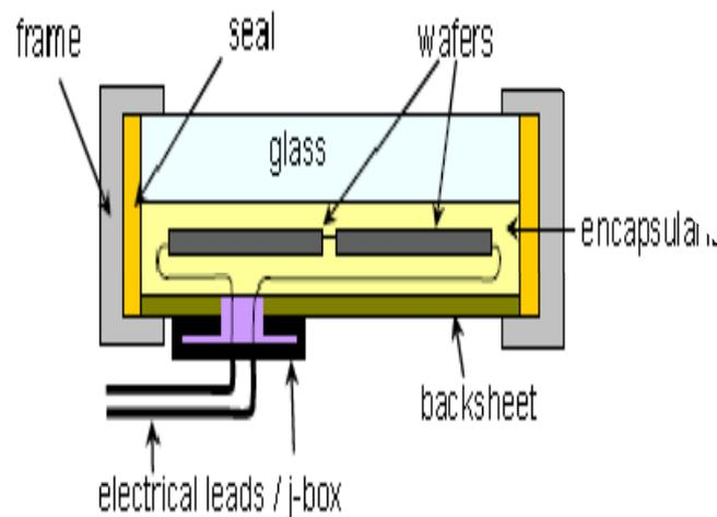
**Figure 10: Typical Packaging of Crystalline Silicon PV Module [1]**
