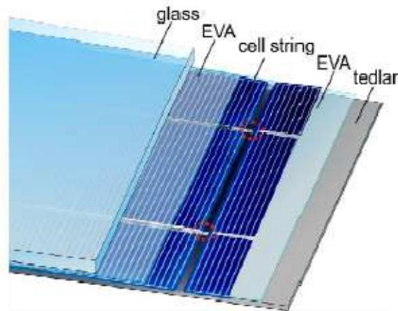
**Figure 6: Schematic of a Typical Build-Up of a Crystalline PV Module (the Red Ellipses Indicate the Critical Areas for the Ribbons) [22]**
