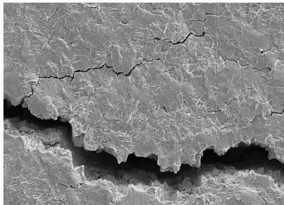
**Figure 7: Ductile Crack Propagates through a Copper Ribbon [22]
