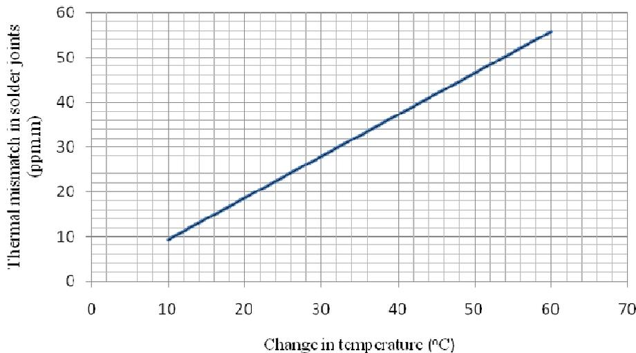
**Figure 14: Effect of Thermal Mismatch in Solder Joint**
