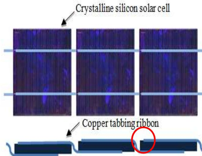
**Figure 2: Crystalline Silicon Solar Cells Interconnected in Series with Tabbing Ribbon: Plan View and Side View**
