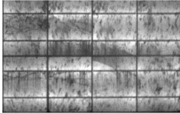
**Figure 9: An Image of a PV Module with Cracked Cells [2]**
