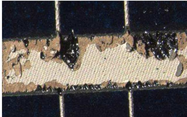
**Figure 8: Failure Mode Due to High Edges and Non-Uniformity Busbar Topology [3]**
