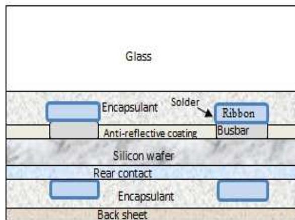
**Figure 4: Schematic of Cross-Section of a Typical Laminated Crystalline Si Solar Cell**
