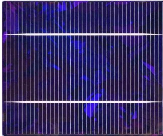
**Figure 1: Typical Crystalline Silicon Solar Cell**
